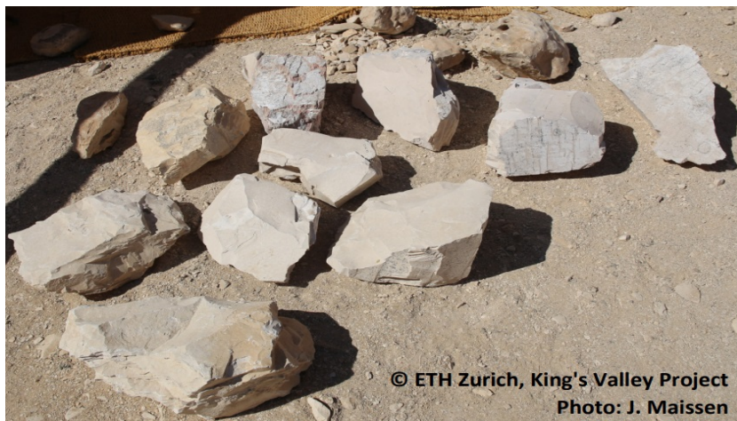
Fig. 21. Collected rock block samples for laboratory rock strength testing. Photo ETH Zurich, Maissen.
