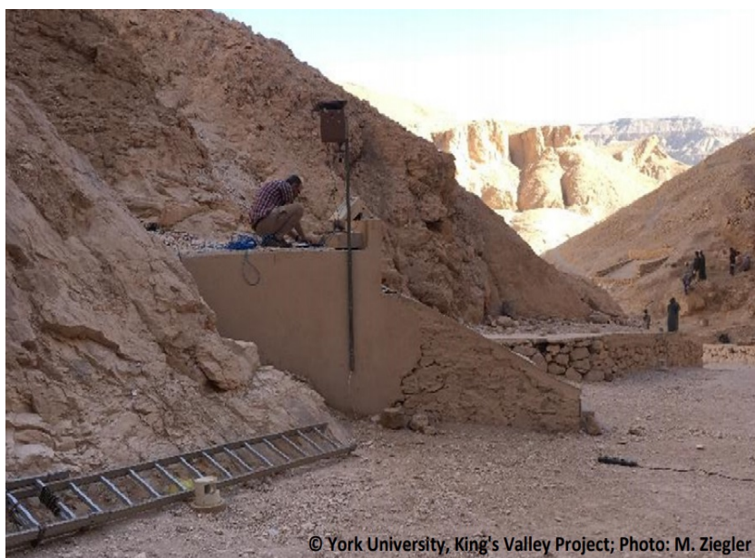
Fig. 23. Picture of the Thermal Station mounted on a pole near the entrance of KV 32 that monitors the temperature of the rock slab above KV 42. Photo ETH Zurich/York University, Ziegler.
