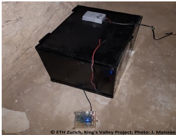
Fig. 22. Metal box with inside battery and voltage converter. On top of the protective box the battery charger can be seen. The Raspberry Shake seismometer is in front of the box. Photo ETH Zurich, Maissen.
